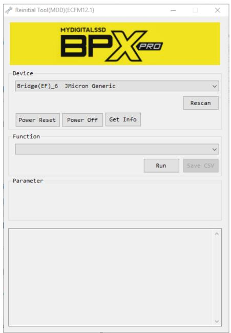
6. Check that the **Device** dropdown menu is set to the **M2X enclosure** by default. If not, select it from the dropdown menu.
